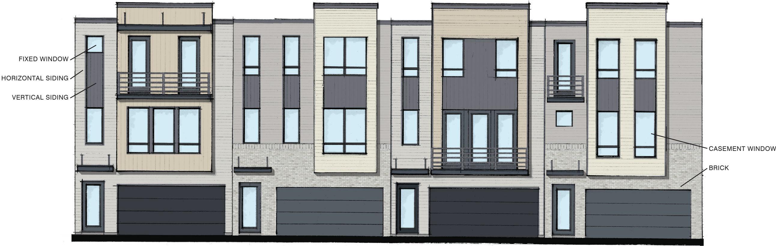
GARRETT I BUILDING STRING :: FRONT ELEVATION
