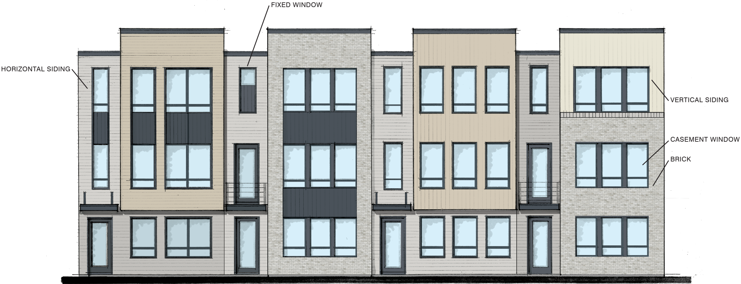
KEMPTON I BUILDING STRING :: FRONT ELEVATION
